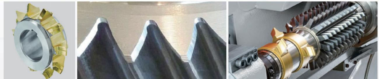
Chamfer cut function for high-quality chamfering after hobbing is supported.
